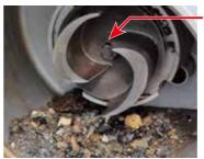
Hex bolt Easily remove with a nut driver.
